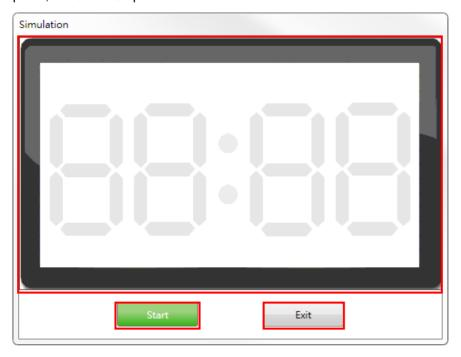
Press the Start button to execute the program from NY8L\_ICE and simulate the LCD by accessing LCD memory data.
